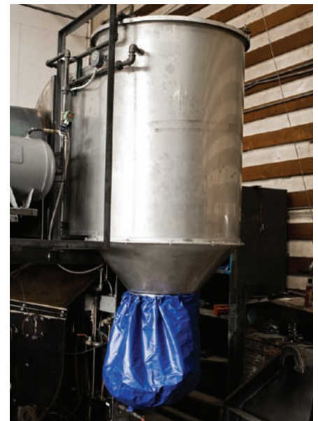
A built-on stainless steel lint collector
